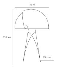
Voltage (V): 230 Volt IP degree: IP20 Maximum bulb wattage (W): 25W Class (Class 1, Class 2, Class 3):
