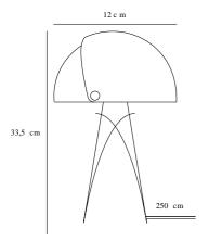
Voltage (V): 230 Volt IP degree: IP20 Maximum bulb wattage (W): 25W Class (Class 1, Class 2, Class 3): Class 2 (Double isolated) Bulb base: E27 Switch placement: On the cable
